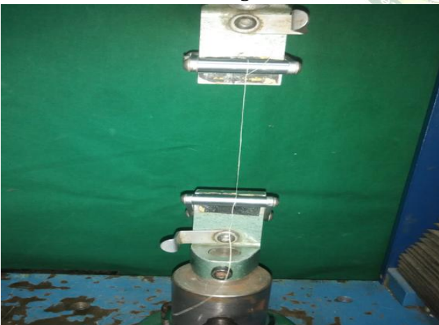
Figure 2: Tensile strength measurement on universal tensile tester
